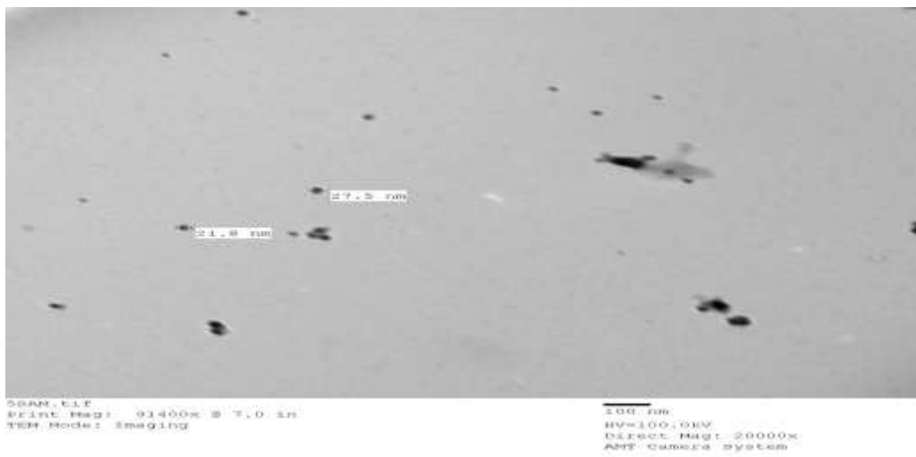
Fig. 5: TEM micrograph at 20,000 times magnification recorded from a drop-coated film of an aqueous solution of AgNPs, showing the spherical shape of the particles and their average diameter of 21.8- 27.5 nm
