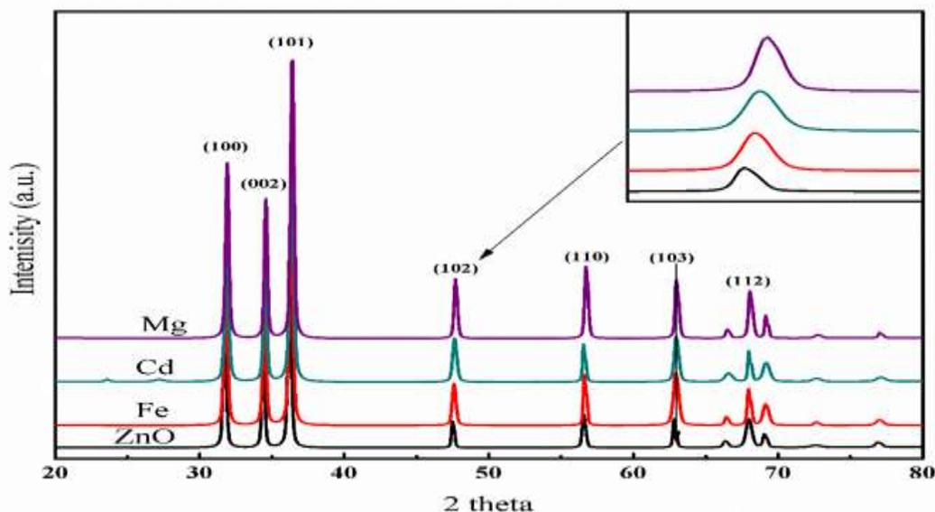
**Fig.1:** XRD patterns of the pure ZnO, and Zn<sub>1-x</sub>TM<sub>x</sub>O NPs
